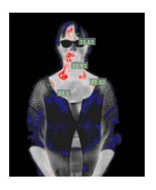
All glass blocks the infrared signal. This image was taken at a distance of 10 feet with a 320 X 240array camera.
